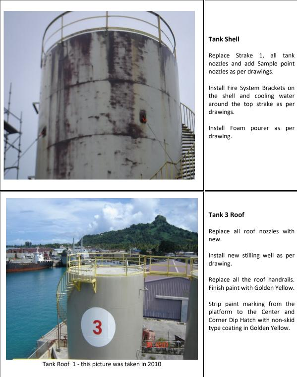
Replace Strake 1, all tank nozzles and add Sample point nozzles as per drawings.
