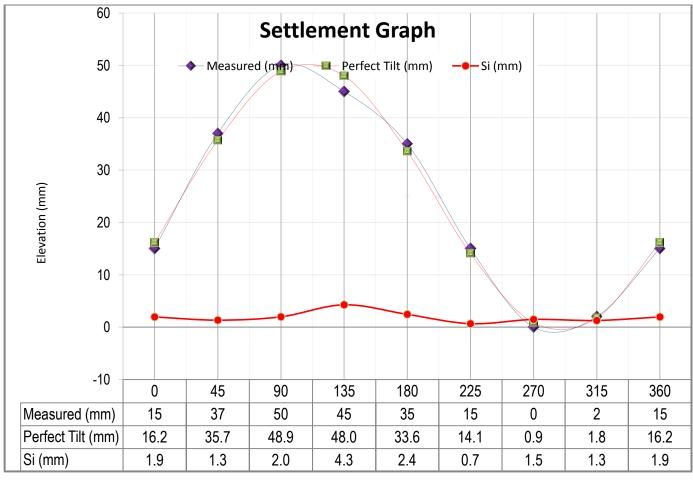
Figure 2-1 : Graphical Representation of Shell Settlement
