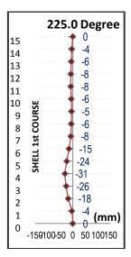
Figure 5-3 : Plumbness Plot for 225 Degree at 1<sup>st</sup> course (Bulging Area).
