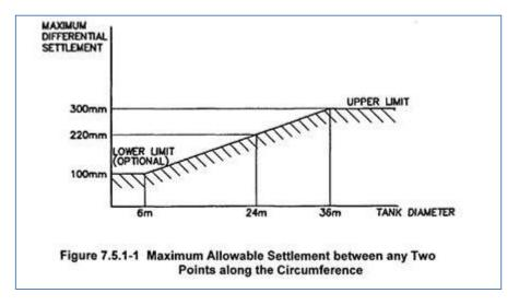
For the 6.096m diameter tank, the maximum acceptable differential settlement is 100.64 mm.
